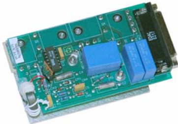
Figure 10.5: Power modulator unit
