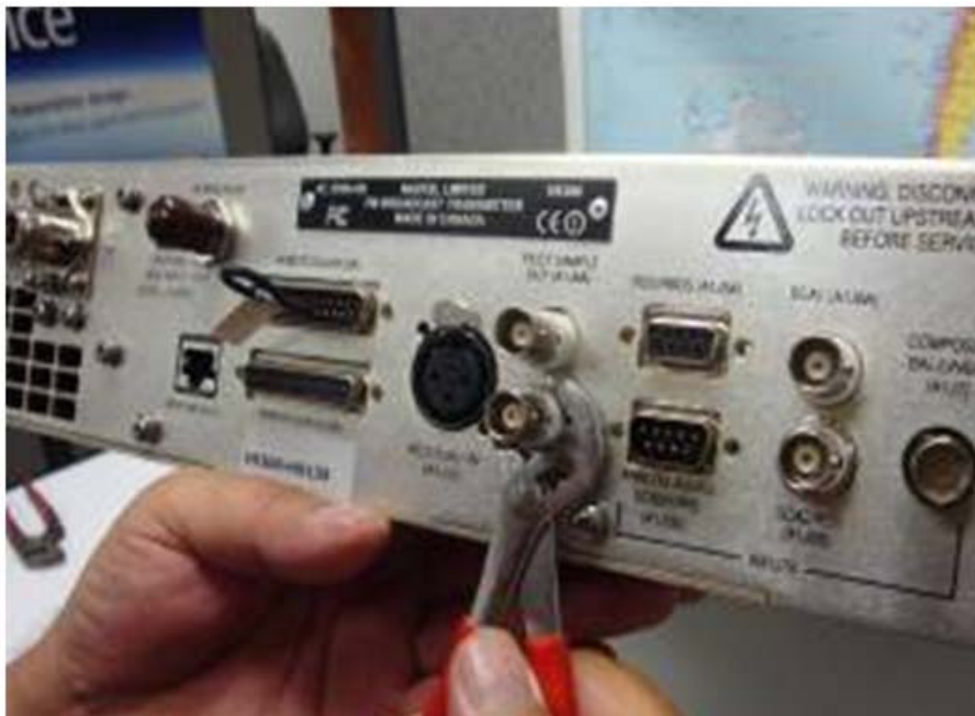
Figure 1.7: Loosening the BNC connector's locking ring
