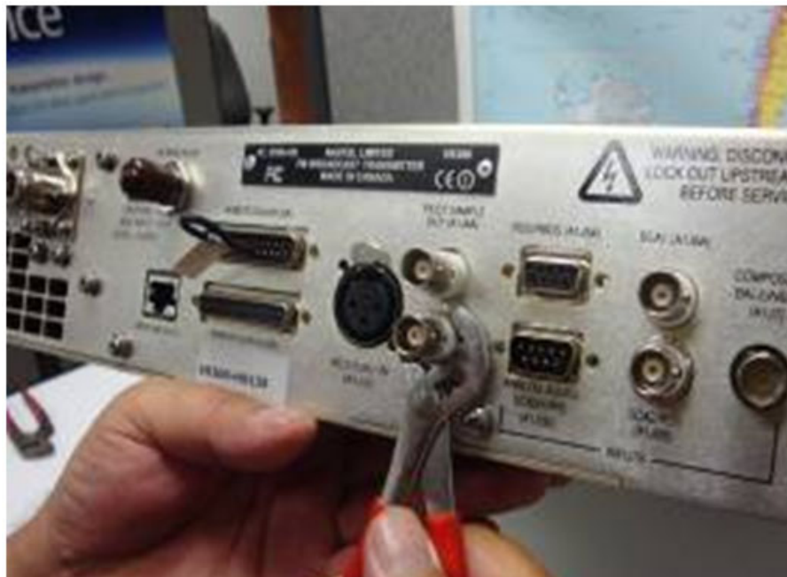
Figure 4.1.26: Loosening the BNC connector's locking ring
