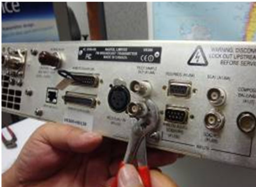
Figure 4.1.26: Loosening the BNC connector's locking ring
