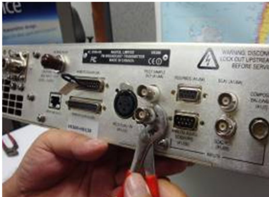
Figure 4.1.26: Loosening the BNC connector's locking ring
